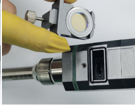
2. Take out the protective lens holder
