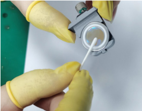
4. Gently wipe the front of the lens with a clean cotton swab or clean cloth dipped in alcohol
