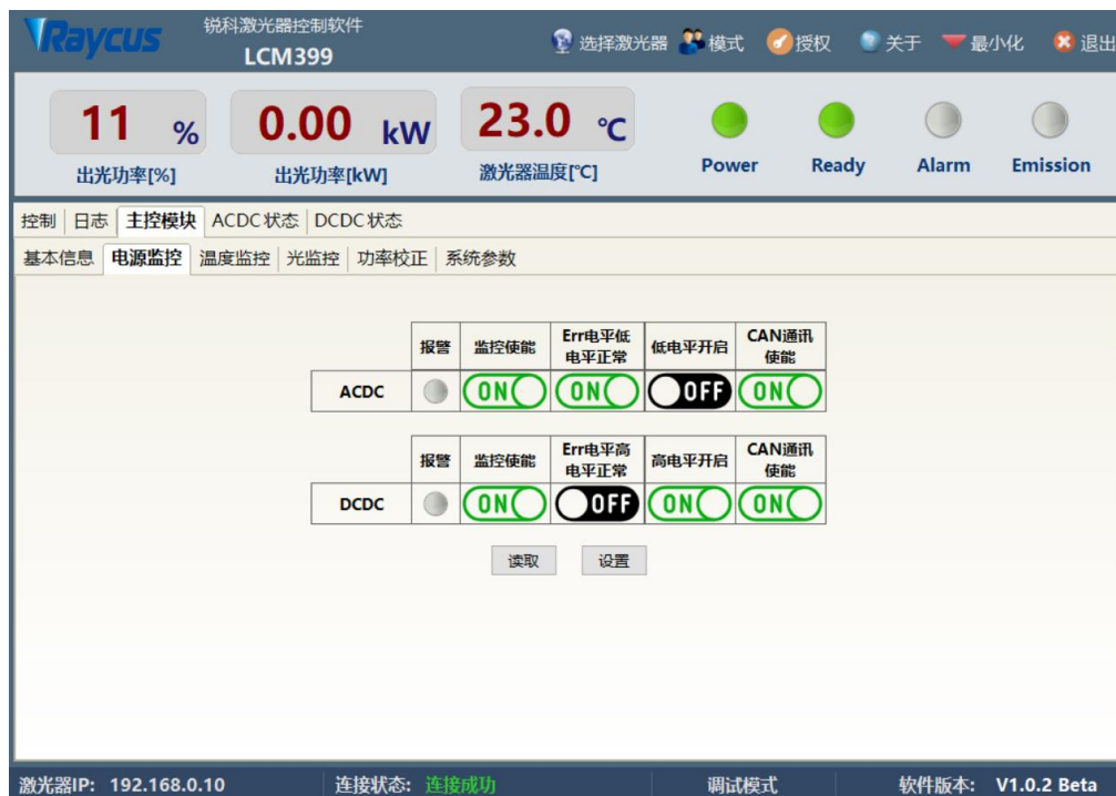
Figure 17 Alarm information interface of main control module
